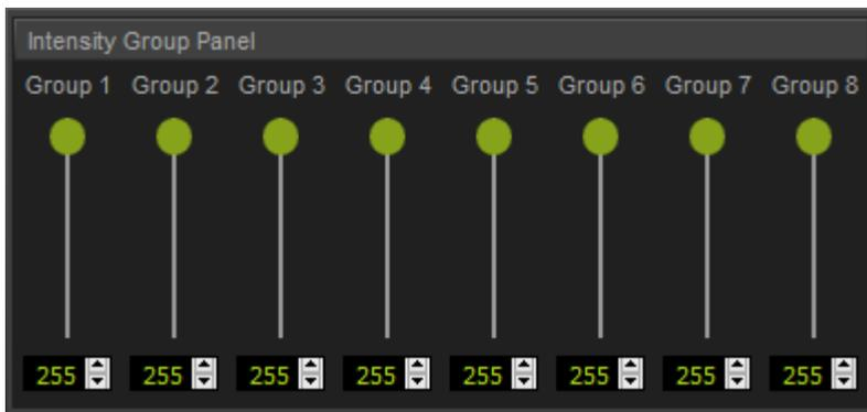
**Faders** Allow you to control the intensity of Intensity Group 1 to 8 with the help of the mouse.
