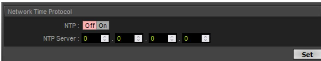
**NTP** Activates [**On**] or deactivates [**Off**] usage of the Network Time Protocol on your device. This protocols can be used to synchronize the clock of your device.
