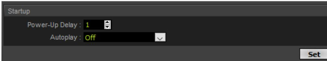
**Power-Up Delay** Defines the wait time before the device fully starts after supplying power to it [in seconds].
