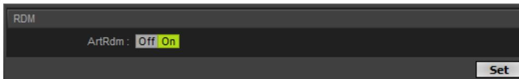
**ArtRdm** Activates [**On**] or deactivates [**Off**] ArtRdm to be able to reply to RDM requests by an RDM controller [for example, MADRIX RADAR] over Art-Net with status and sensor data. MADRIX AURA mainly provides data regarding:
