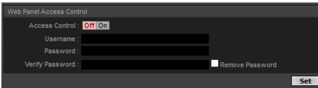
**Access Control** Allows you to restrict access to the MADRIX AURA web configuration by requiring a login with username and password if set to **On**. Otherwise, the device's web configuration can be accessed without any login credentials [**Off**].
