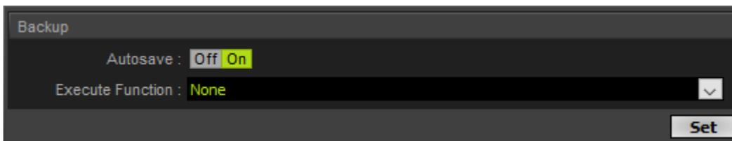
**Autosave** Activates [**On**] or deactivates [**Off**] automatic saving for your device. This saves the settings and configuration automatically to SD card when using Set in the Cue List, Timers, Channel Mask, and Remote. The default setting is On.
