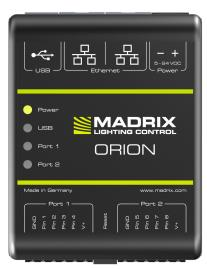
Each input can be separately set as Analog-IN, Digital-IN, Counter, and other useful functions in the web configuration page. Data is then send over network with Art-Net or Streaming ACN (E1.31). The device also features 2 separate network ports to linearly daisy-chaining several devices together for better cable management.
